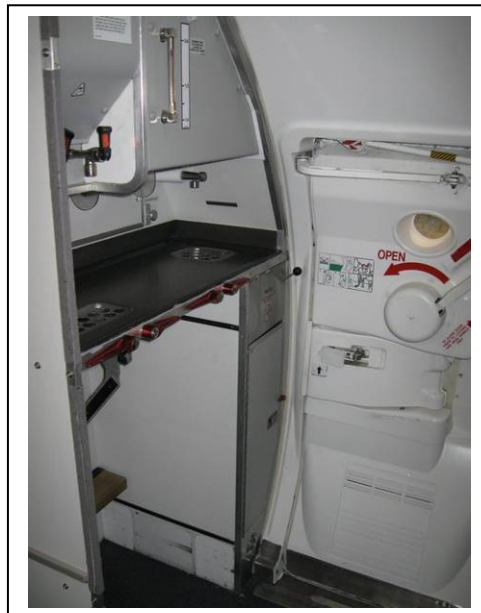
G5 Galley – Rear RHS, Aft Facing Composed of G1 + extension - 2 carts - 50L water tank and boiler - 4 SU's - Work counter - Trash bin - Misc stowage
