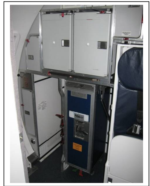
G3 Galley* – Rear RHS, Fwd Facing - 4 carts - 1 SU - 2 Ovens - Work counter - Trash bin - Misc. stowage
